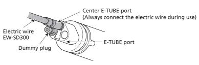
• Be sure to attach the dummy plugs to any E-TUBE ports that do not have electric wires connected to them.
